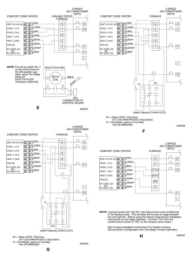
Fig. 20—Typical Wiring Diagrams (Furnace with Air Conditioner) Continued
